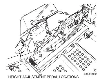
Figure 4-8. Height Adjust Pedal Locations
